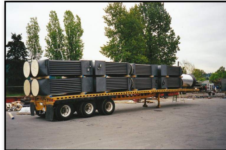
Type 321 stainless acid gas heater bundles
